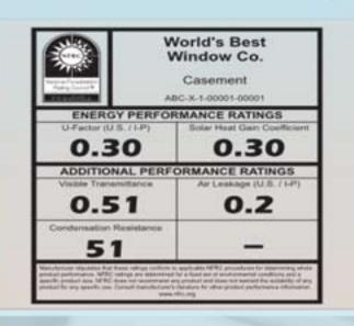
U-factor measures how well a product prevents heat from escaping a home or building. U-factor ratings generally fall between 0.20 and 1.20. The lower the U-factor, the better a product is at keeping heat in. U-factor is particularly important during the winter heating season. This label displays U-factor in U.S. units. Labels on products sold in markets outside the United States may display U-factor in metric units.
